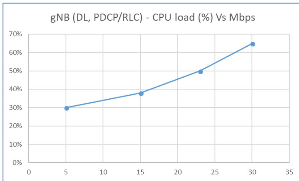
**Figure 3-8: CPU load versus the traffic load (in Mbps) that the higher layers serve (eMBB slice, gNB part, DL flow)**
