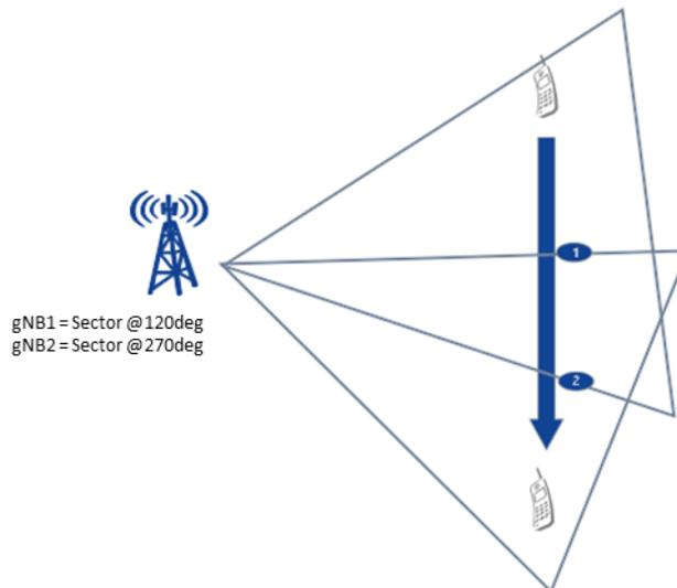
**Figure 3-10: Illustration of multi-connectivity approach implemented in the Smart Sea Port testbed**
