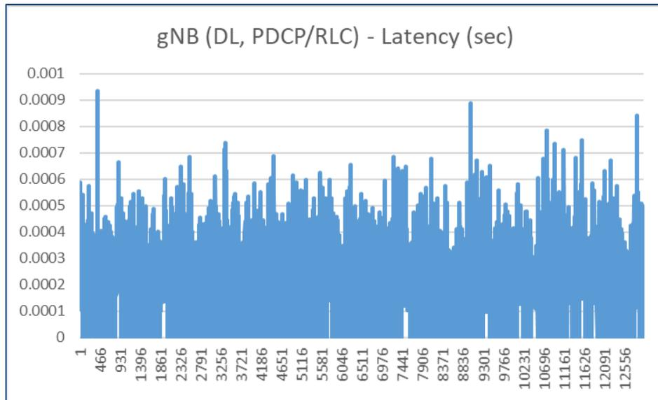
**Figure 3-9: Time needed for the higher layers processing per received packet (eMBB slice, gNB part, DL flow)**
