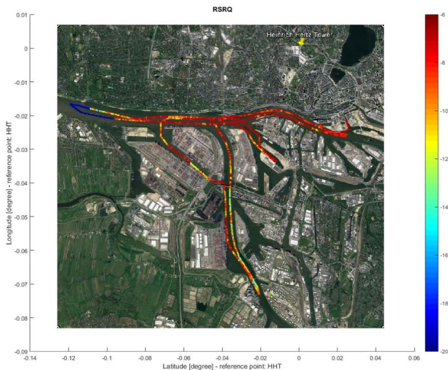
*Figure 5-12: RSRQ measurement results within Hamburg port area*
