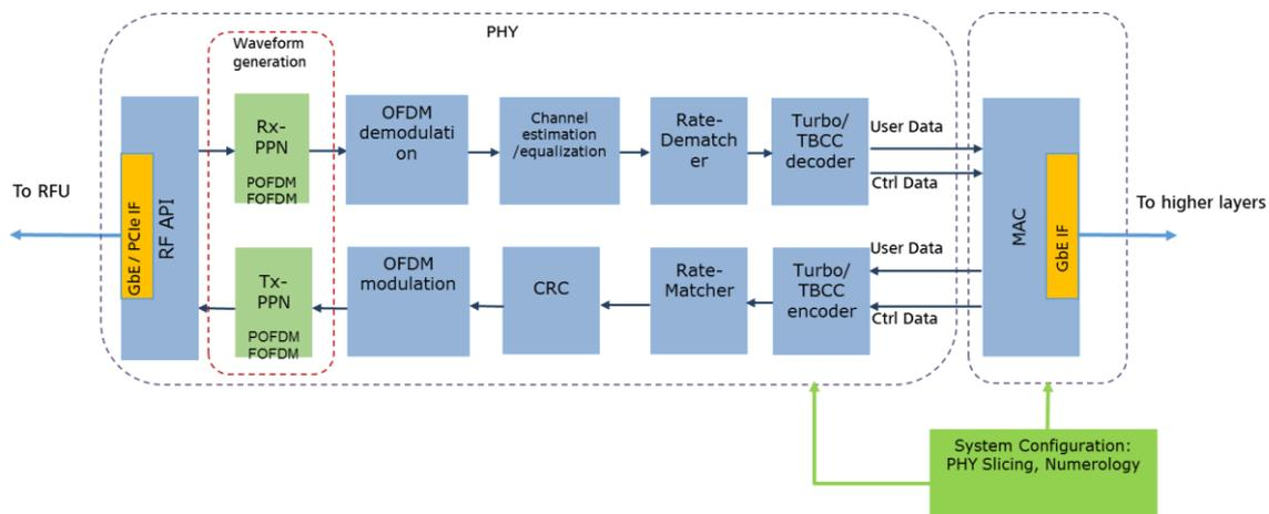
Figure 5-13: Block diagram of the baseband unit (PHY layer)
