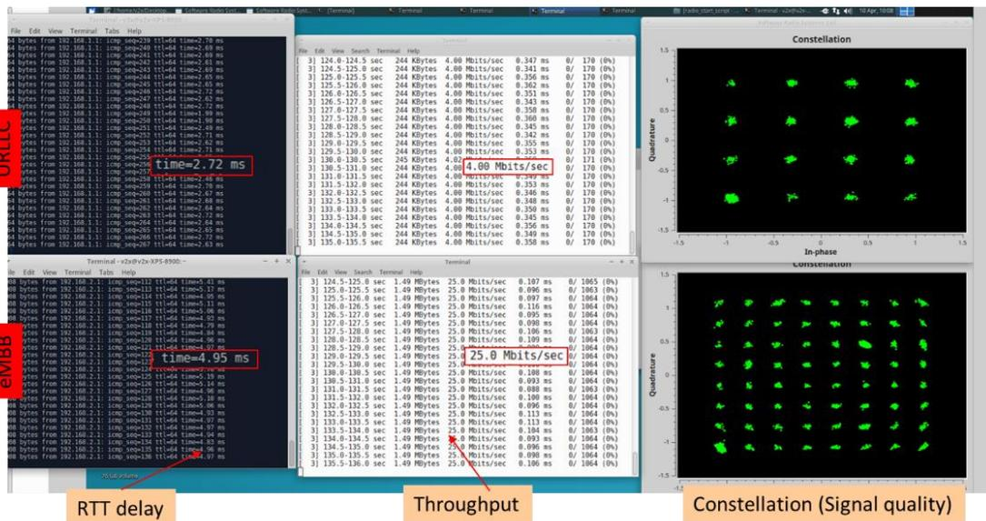
Figure 3-6: Throughput and latency measurement using IPERF
