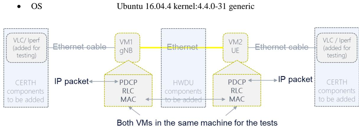
**Figure 3-7: Illustration of the set up used for the higher layer’s tests**
