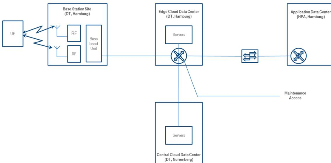
*Figure 5-1: Physical components of the Smart Sea Port testbed*
