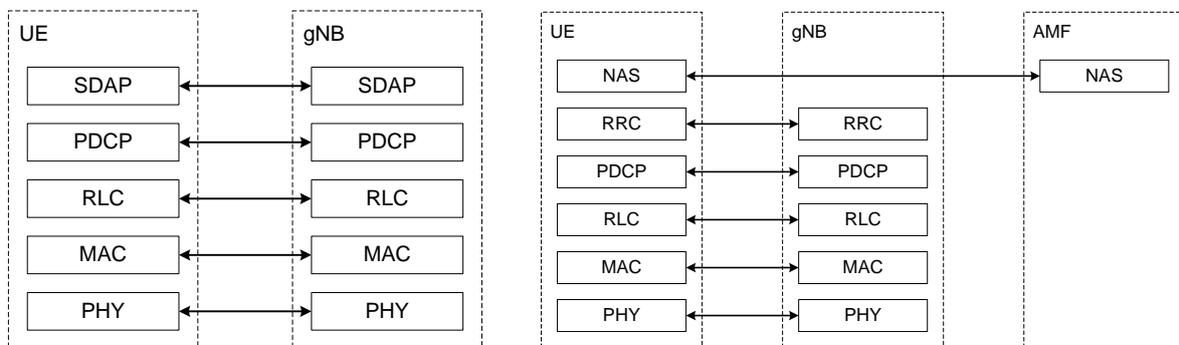
Figure 5-15: a) user plane protocol stack (left), b) control plane protocol stack (right)
