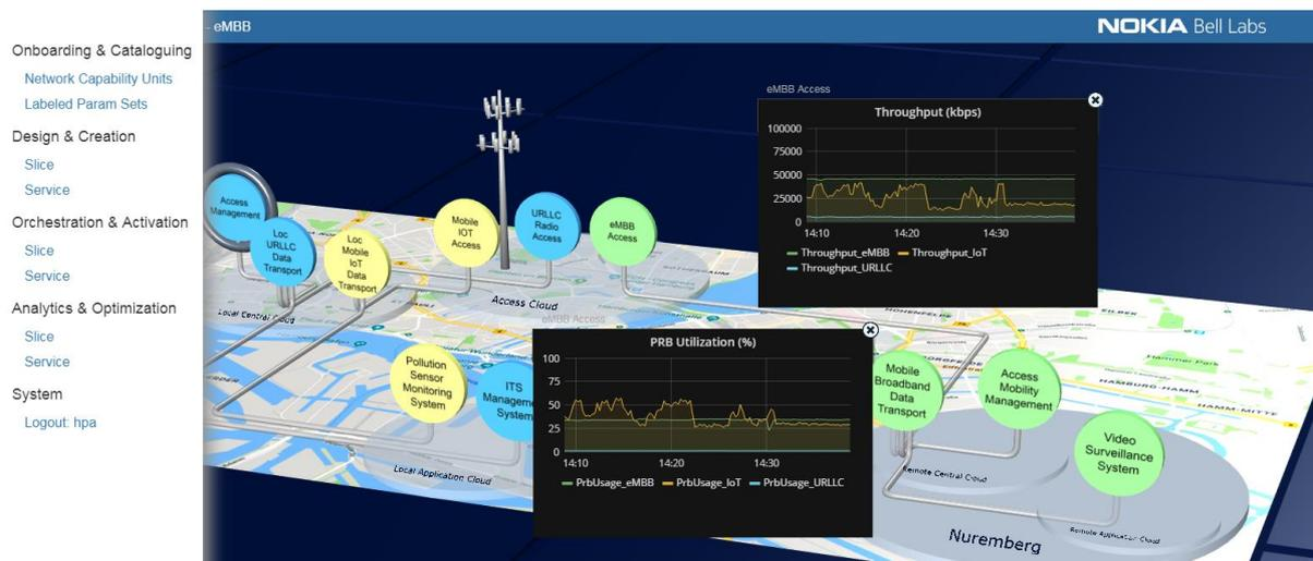
Figure 5-5: Screenshot of GUI used to control the network slice lifecycle management
