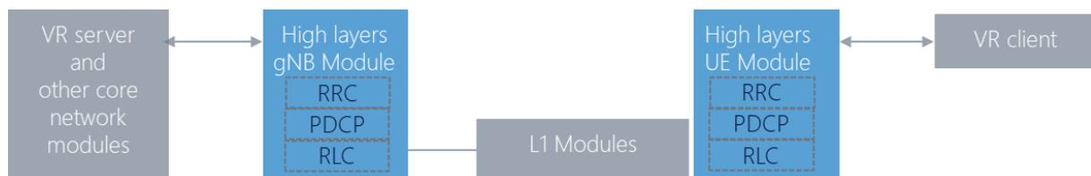
Figure 5-16: High layers' modules
