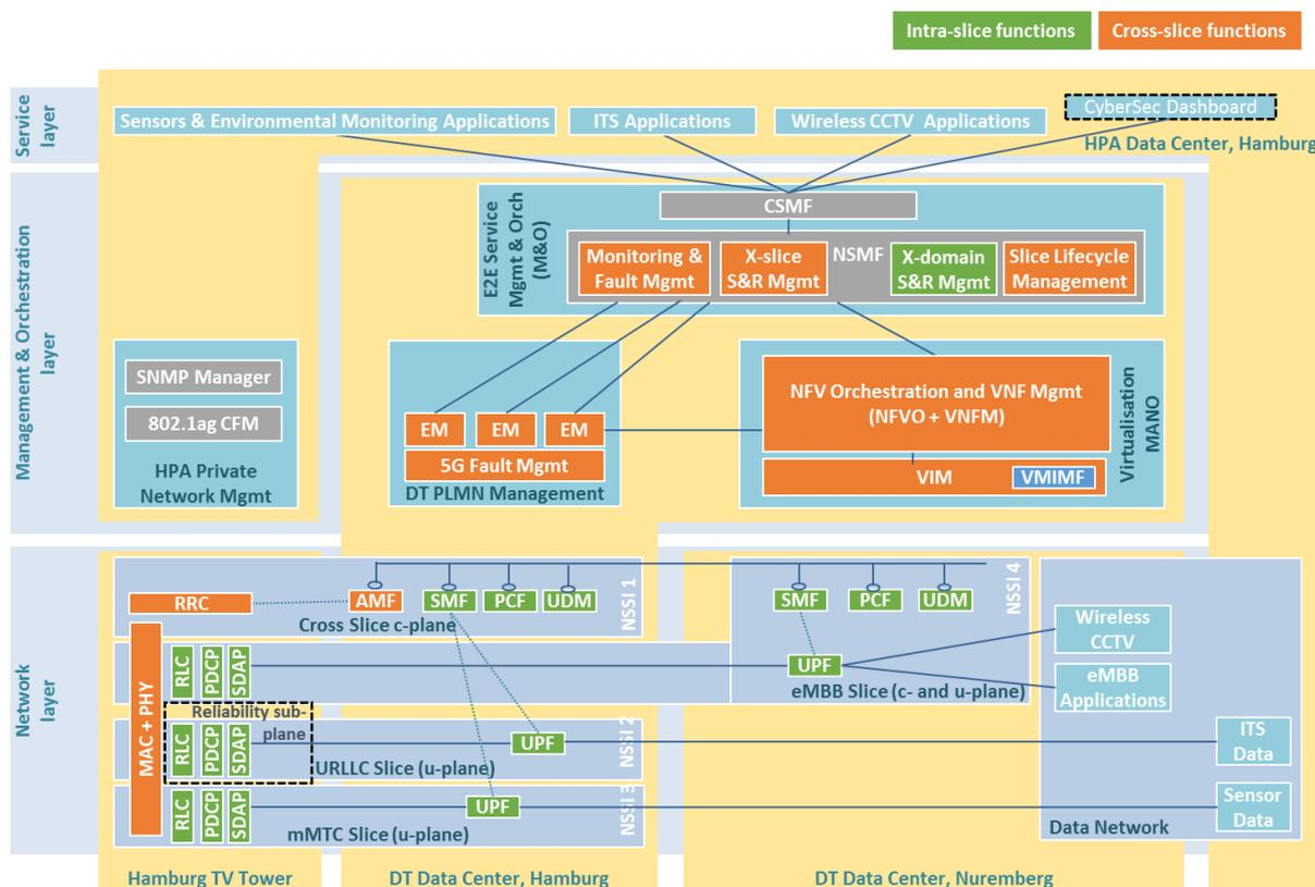
Figure 3-2: Targeted functional architecture for the Smart Sea Port testbed [5GM18-D22]
