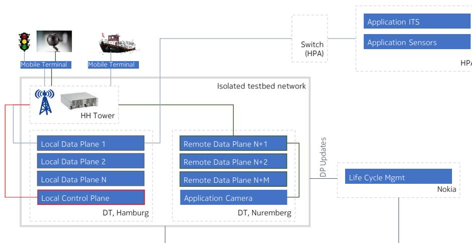
Figure 5-4: Logical deployment of Smart Sea Port testbed
