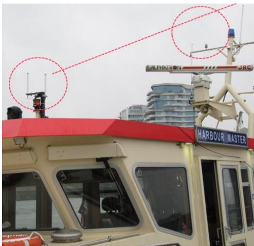
**Figure 5-9: Antenna and sensor-box installation points on barge**
