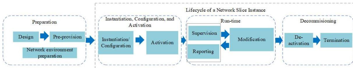
**Figure 3-14: Lifecycle of a network slice instance [3GPP18-28801]**
