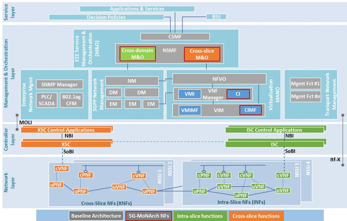
**Figure 3-1: Initial high-level functional view of overall 5G-MoNArch architecture [5GM18-D22]**
