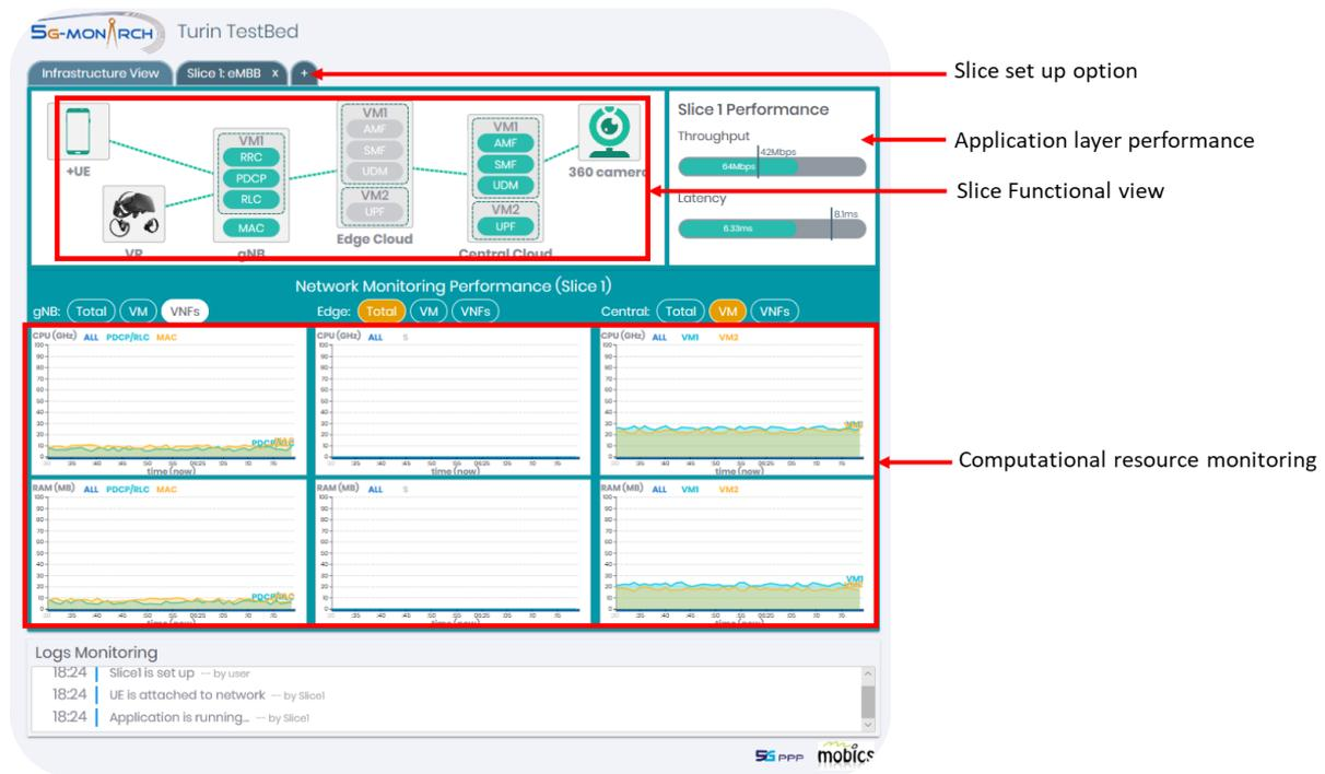
Figure 5-32: Basic screen of the GUI under development for the Touristic City testbed
