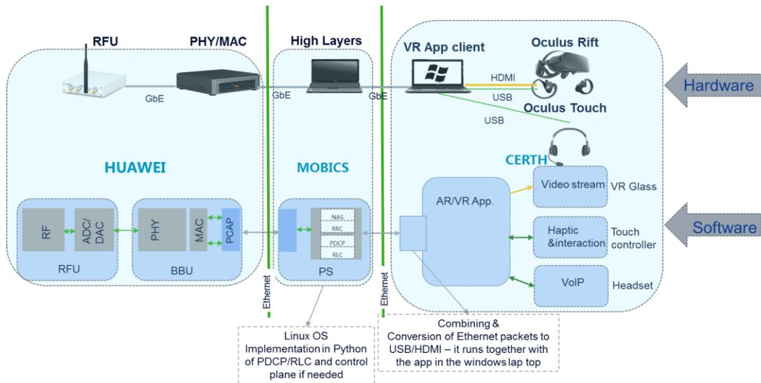
Figure 5-28: Interfaces between different hardware/software modules at UE side
