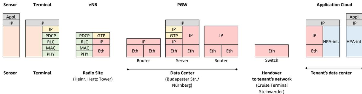
**Figure 5-2: Simplified user plane protocol structure for communication between UEs and application servers.**
