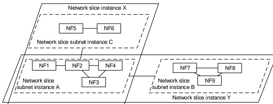
Figure 3-4: NSI X and Y composed by NSSI A, B and C [3GPP18-28801]
