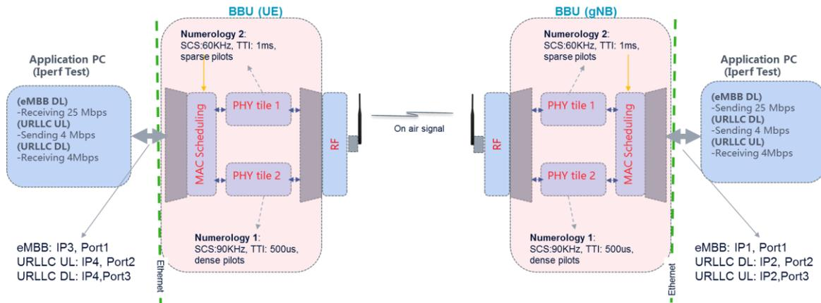
Figure 3-5: PHY with two bandwidth partitions with different numerologies
