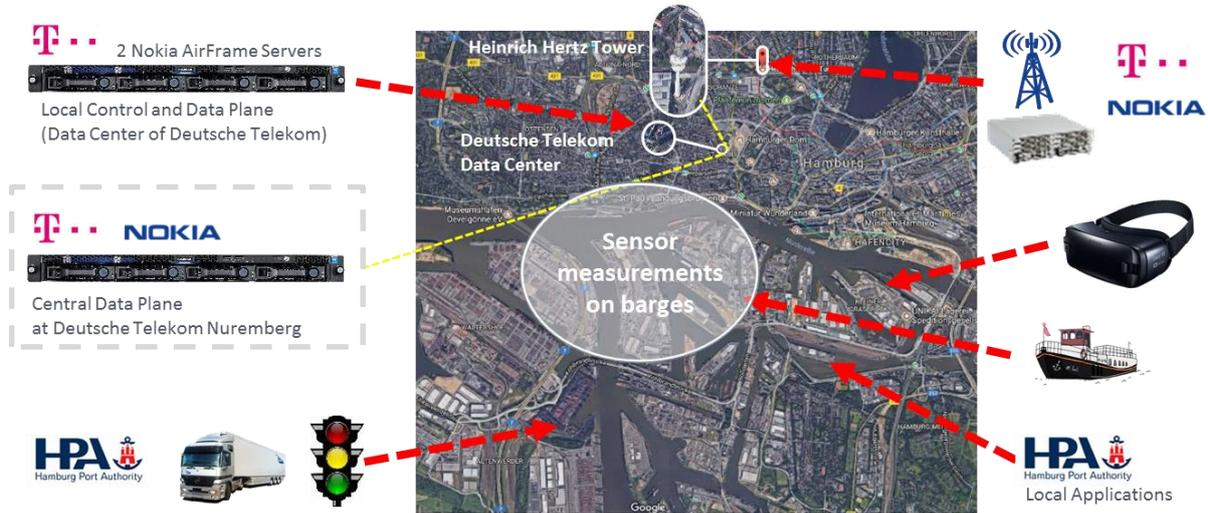
Figure 5-3: Physical deployment of Smart Sea Port testbed
