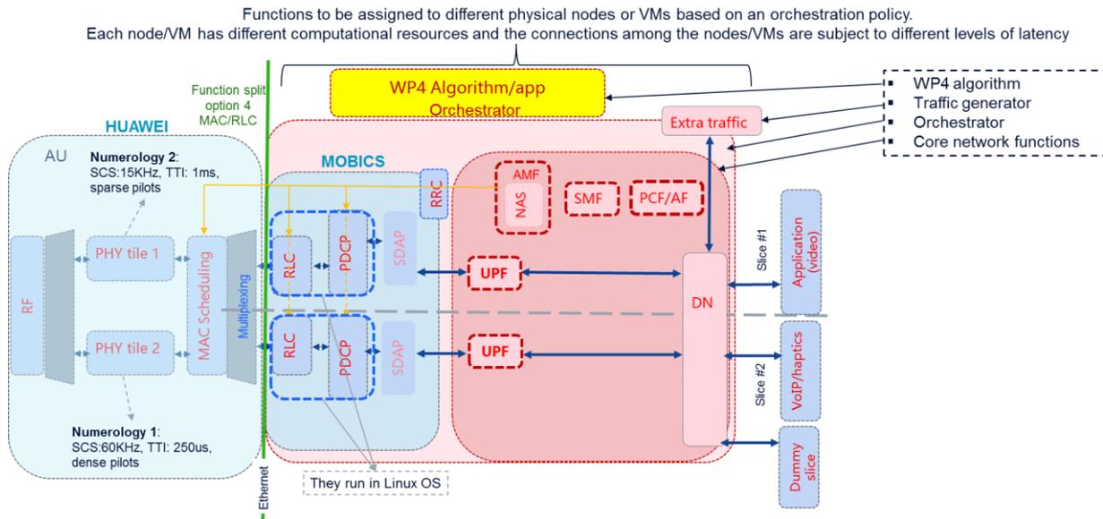
**Figure 5-31: Software modules and interfaces at the network side**
