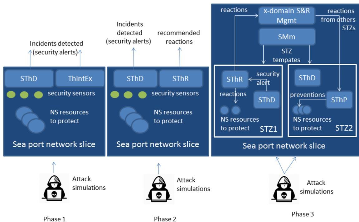
**Figure 3-12: Security mechanisms strategy for validation over the Smart Sea Port testbed [5GM18-D31]**
