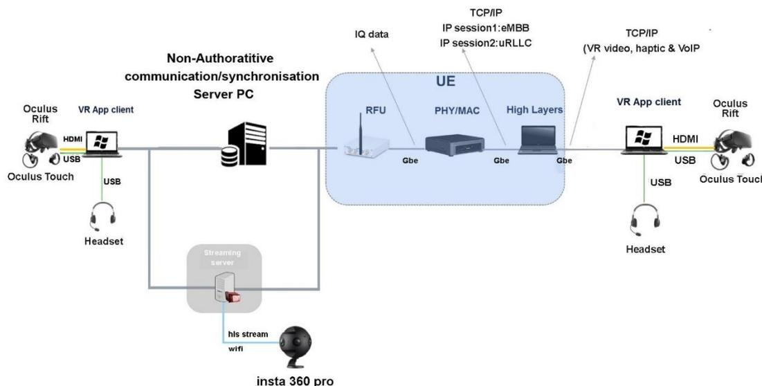
***Figure 5-17: Physical connection of video streaming server***
