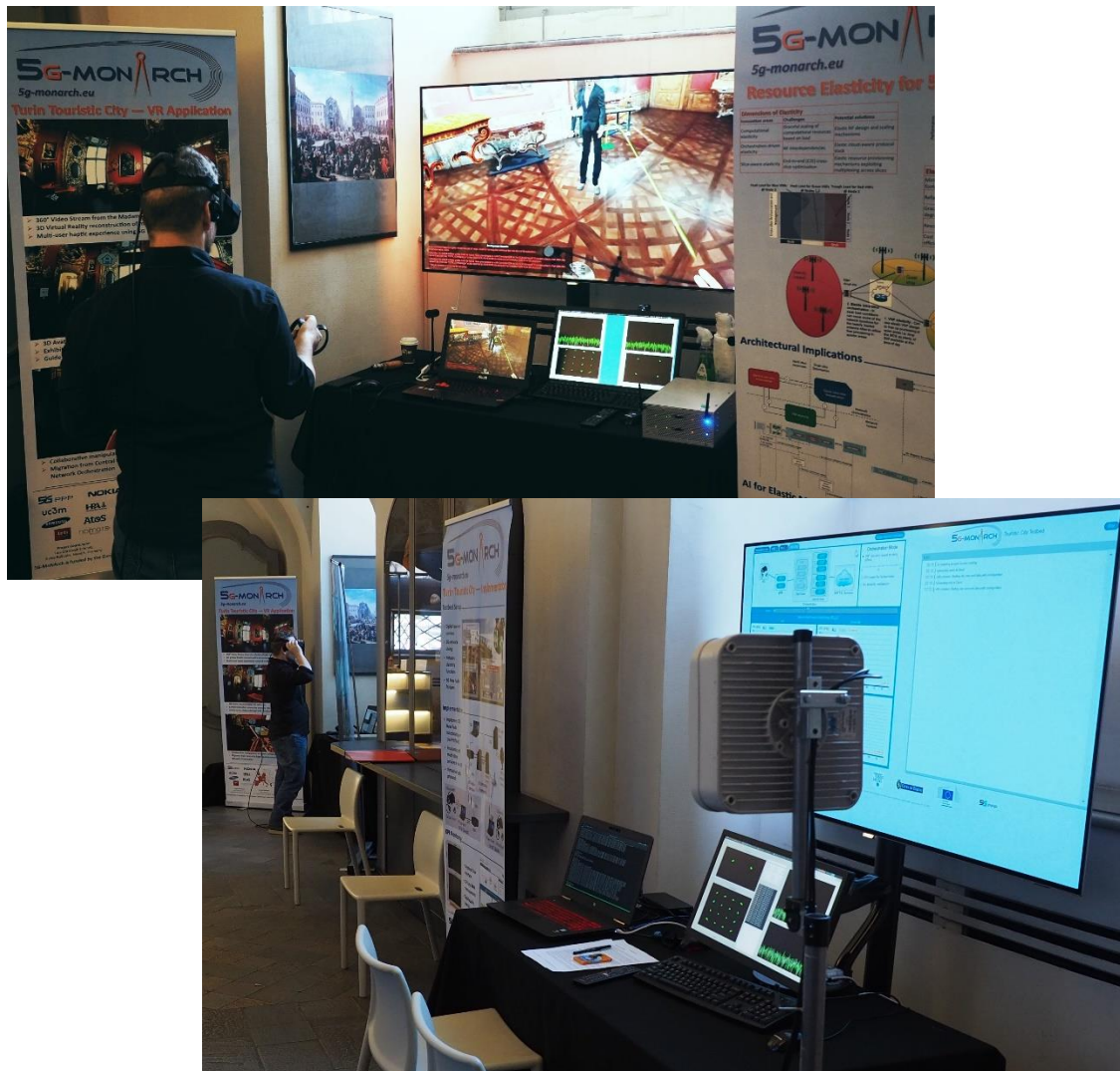
Figure 9: Turin Touristic City testbed life demonstration with interactive Virtual Reality application running (upper); full setup at bookshop in Palazzo Madama with radio base station and monitoring GUI (lower)
