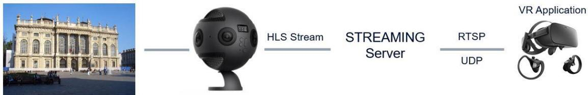
**Figure 5-18: Physical connection of Insta360 Pro**
