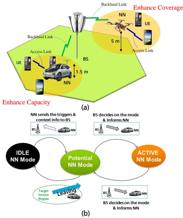
Figure 3 5G use case with unplanned dynamic small cells.
