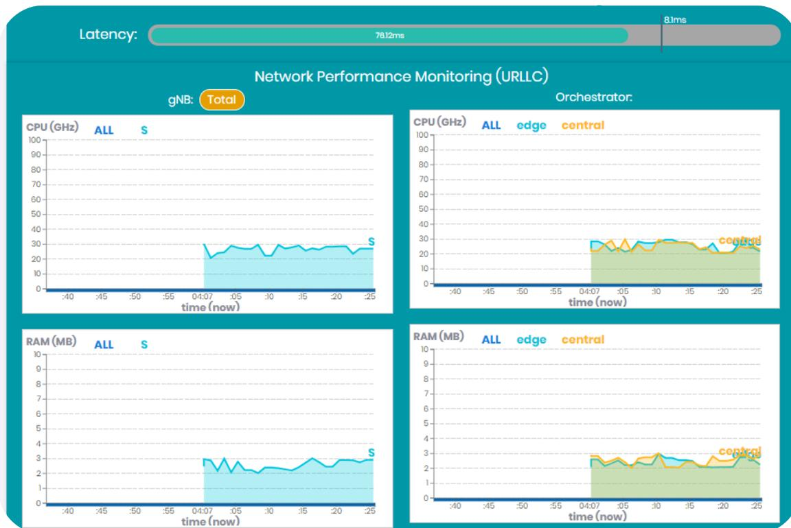
Figure 4-32: GUI with the KPIs of the Touristic City testbed (latency and CPU/RAM usage)
