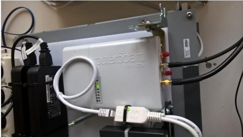
**Figure 3-4: Mikrotik RouterBoard used in the testbed**
