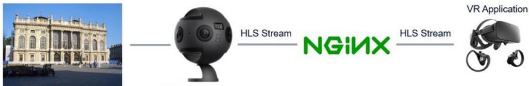
**Figure 4-12: Logical connection of Insta360Pro**
