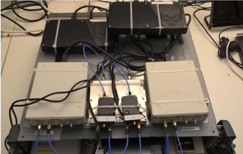
**Figure 3-6: Picture of one multi-connectivity device used in the testbed**
