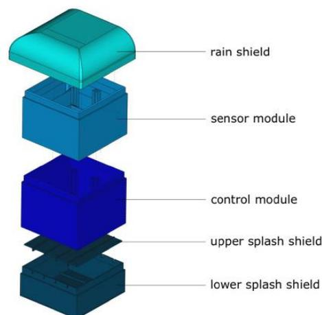
**Figure 3-7: Sensor-Box design**
