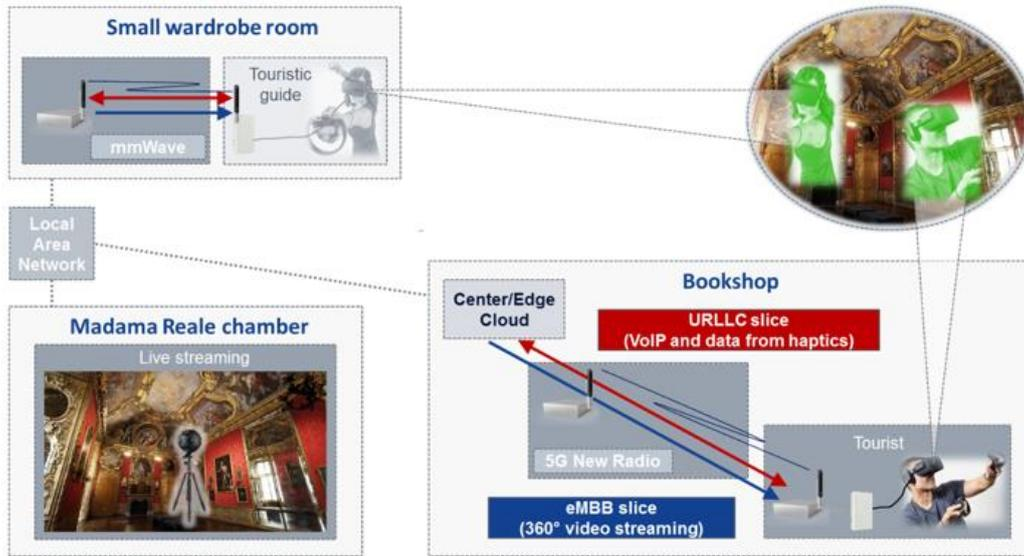
Figure 4-1: High level implementation of the Touristic City testbed
