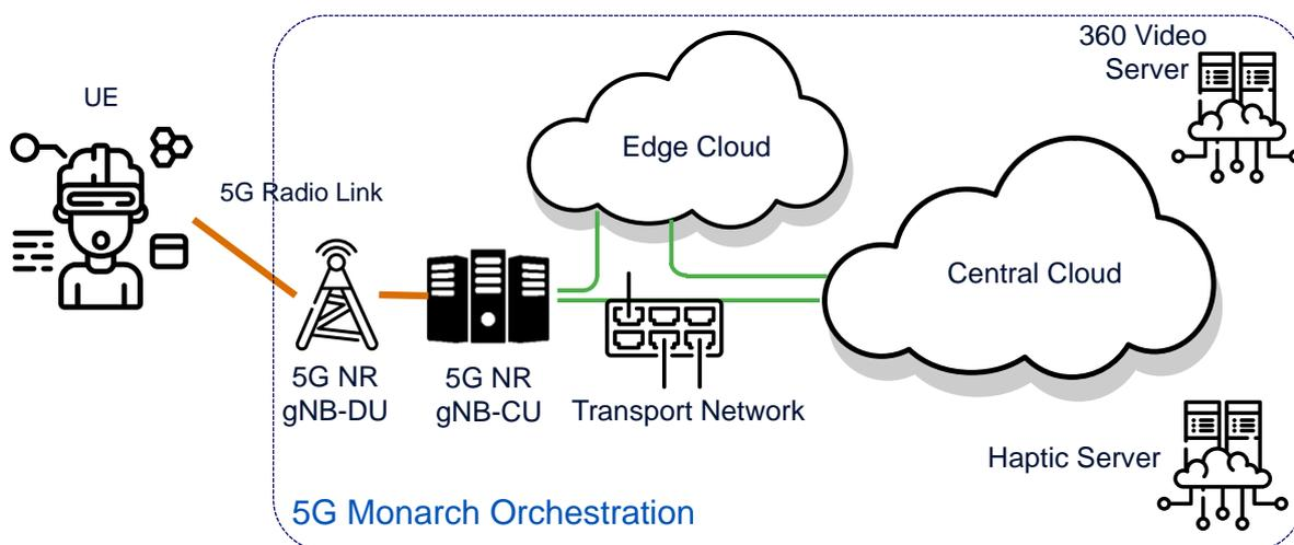
**Figure 4-5: Testbed HW and SW setup**
