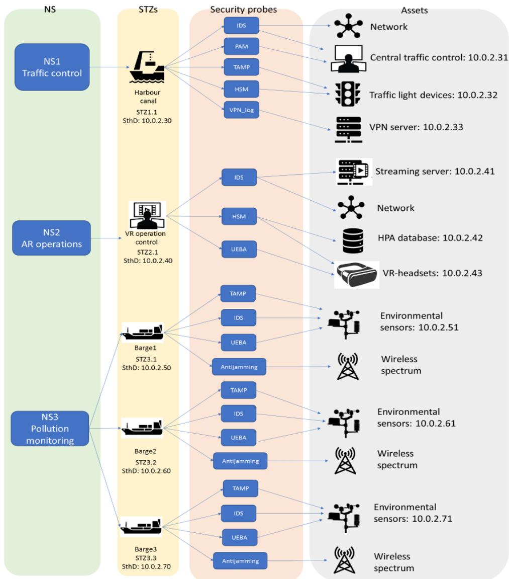
Figure 3-27: Deployment of SthD simulated assets and probes in the testbed
