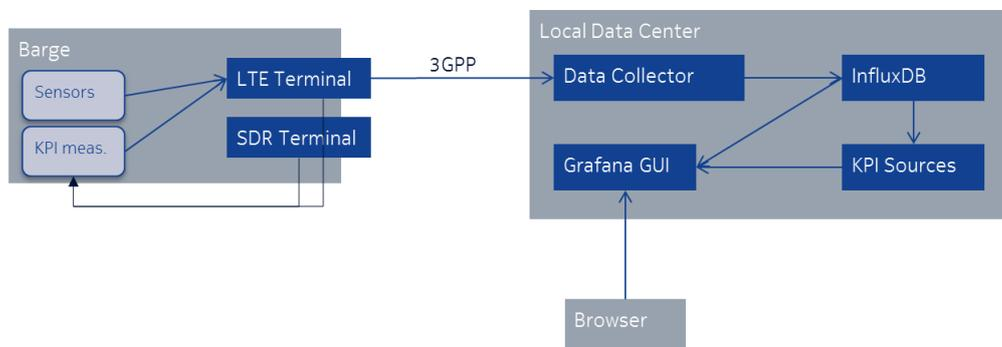
*Figure 3-17: Setup of performance monitoring in Smart Sea Port testbed*
