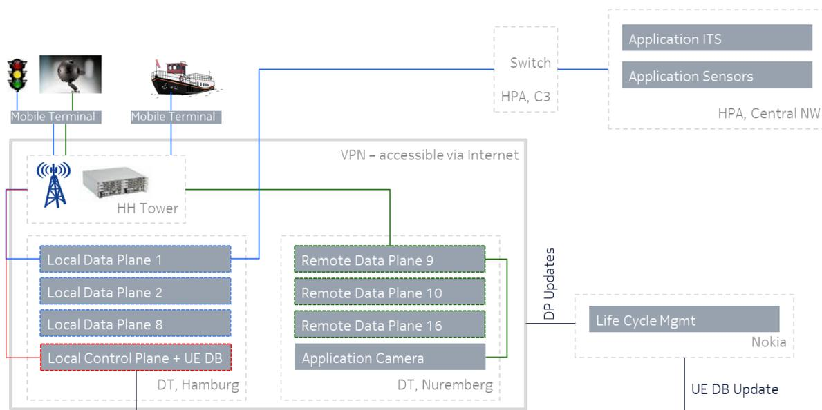
**Figure 3-11: Logical deployment of the Smart Sea Port testbed**
