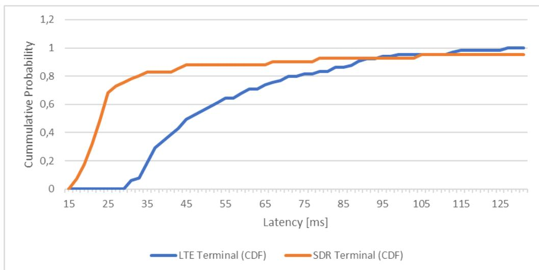
**Figure 3-23: CDF of average round-trip latency of LTE and SDR terminal during handover**
