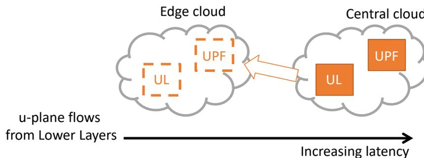
Figure 4-33: The VNF relocation scenario (c-plane functions are omitted for the sake of clarity)
