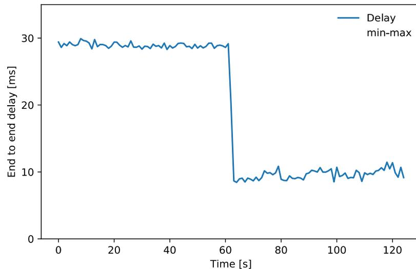
**Figure 4-34: The overall E2E delay (UE-UPF)**
