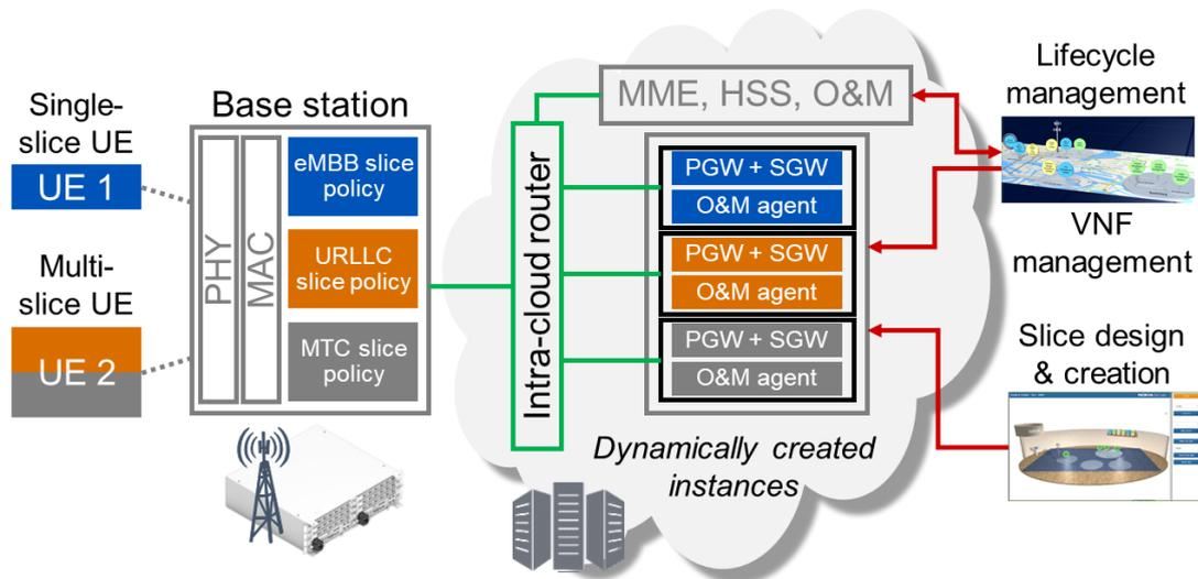
*Figure 3-16: Slicing of network layer functionality in the Smart Sea Port testbed*
