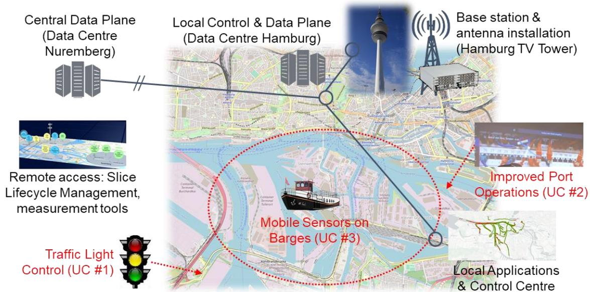
*Figure 3-15 : Physical deployment of the Smart Sea Port testbed*
