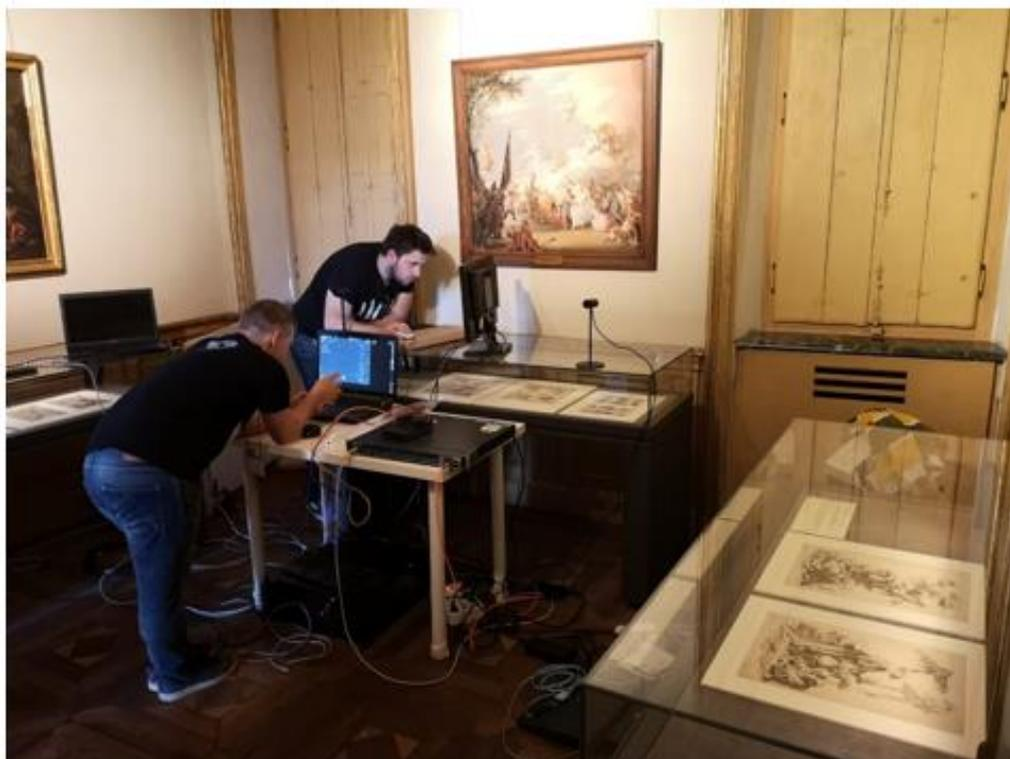
*Figure 7-18: Installation in the Small Wardrobe (360° video server, VR application server and VR client of the first user)*
