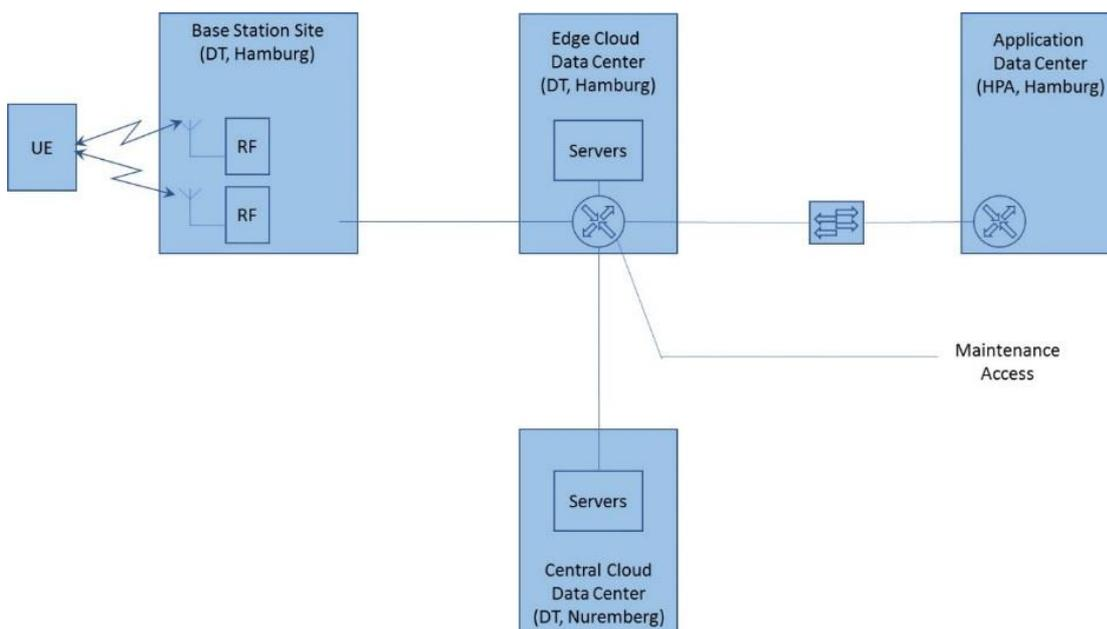
Figure 3-14: Physical components of the Smart Sea Port testbed
