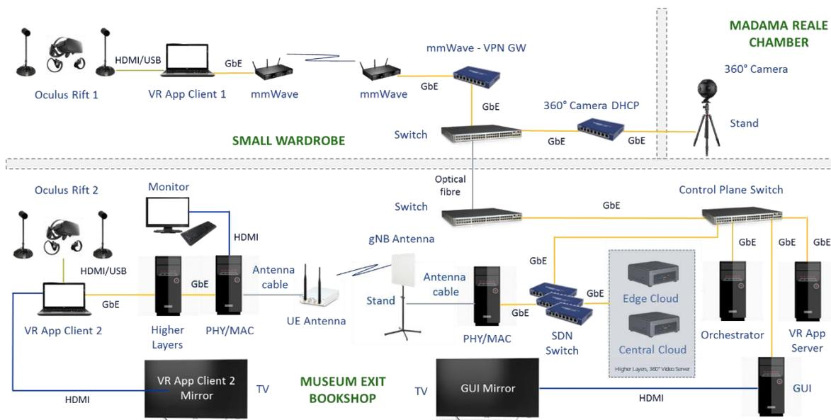
Figure 4-2: Final Touristic City testbed setup scheme
