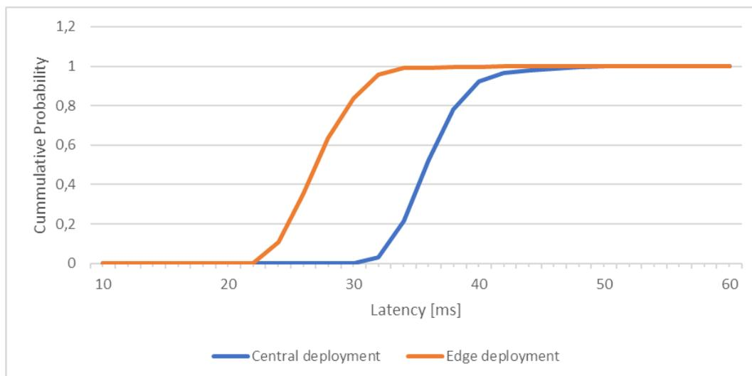
**Figure 3-20: Round-trip latency towards centrally and locally deployed UPF**
