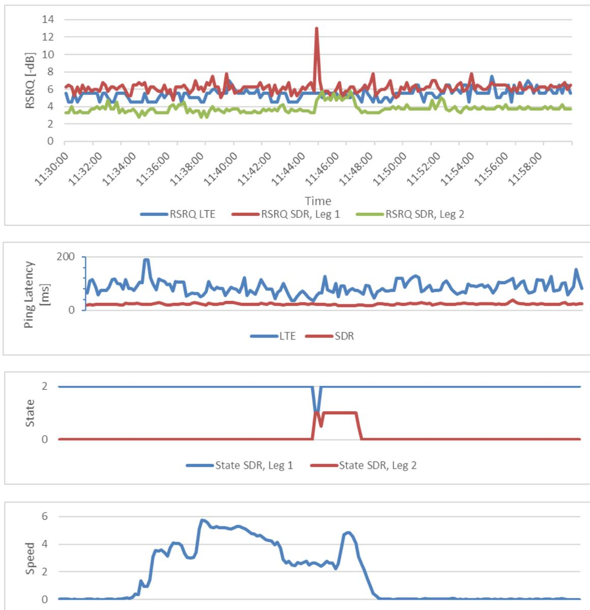
Figure 3-22: Grafana dashboard output for the tracking the performance of SDR terminals
