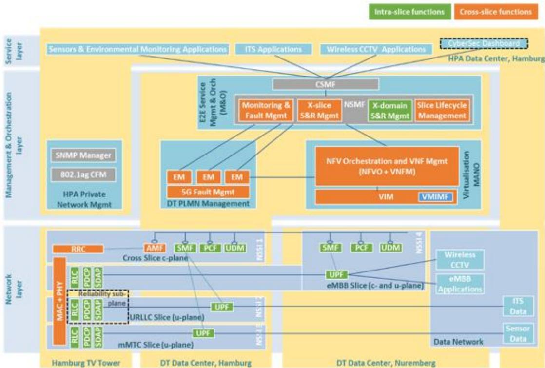
Figure 3-10: Targeted functional architecture for the Smart Sea Port testbed [5GM18-D51]
