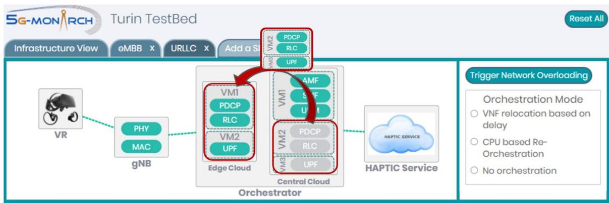
Figure 7-16: PDCP, RLC and UPF relocation in the Touristic City testbed
