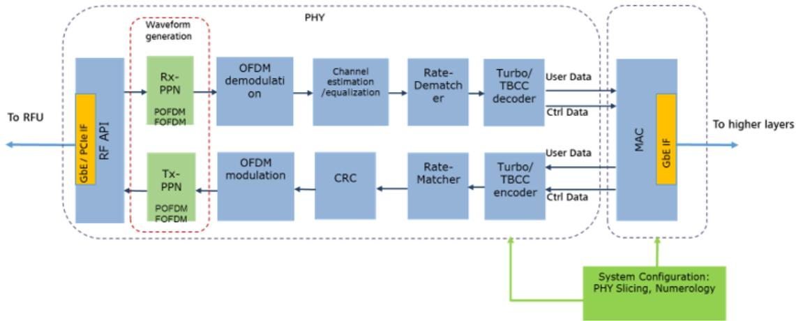
**Figure 4-4: Block diagram of the baseband unit (PHY layer)**
