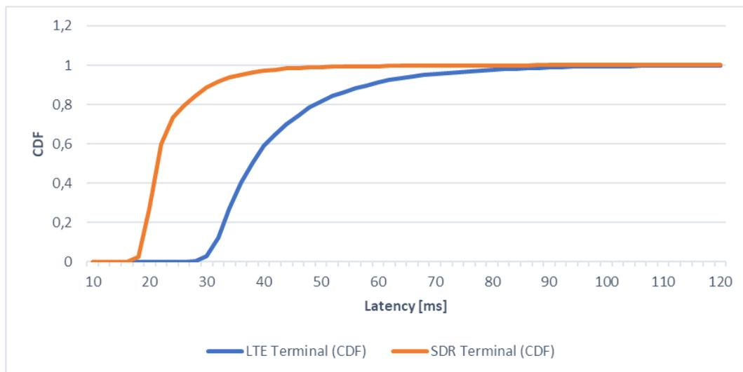
**Figure 3-19: CDF of round-trip latency of LTE terminals compared to self-developed SDR device**
